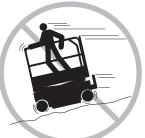
Limit travel speed according to the condition of the ground surface, congestion, slope, location of personnel, and any other factors which may cause collision.
